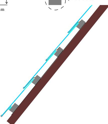
DS\_SK020. Screwed in the laths as shown in the drawing, these hold the CFR modules clamped to the laths at the top and bottom. 4 brackets are installed per unit, but more can be fitted if required. DS\_SK020 can be painted to the desired color and milled into the laths to reduce the height.
